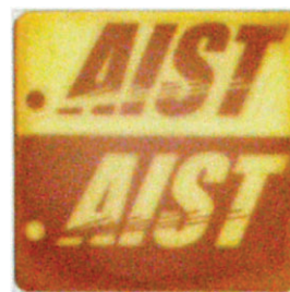
Fig. 2 A photograph of a polymer film (22 mm \times 22 mm) having PNI (3 wt%) dispersed in polycarbonate after 405 nm light irradiation through a photomask. The irradiated area turns to brown.
